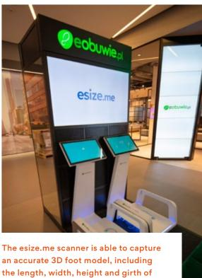
an accurate 3D foot model, including the length, width, height and girth of the foot. The 3D image and precise foot dimensions are displayed on a touchscreen device, where you can see the detailed model and dimensions data. The scanning process takes a few seconds and is free of charge
